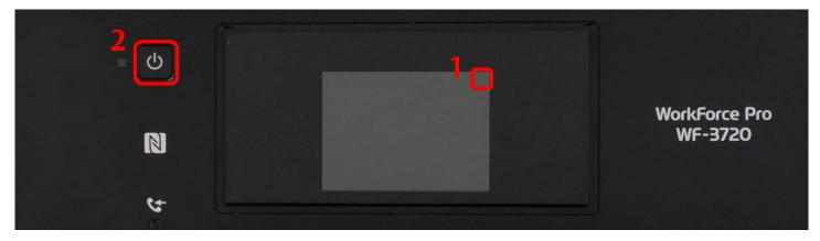
Please note that the inscription on the display must be in white font. If the text is red, this is an incorrect mode, turn off the printer, and then repeat the procedure for entering the printer in firmware mode.
