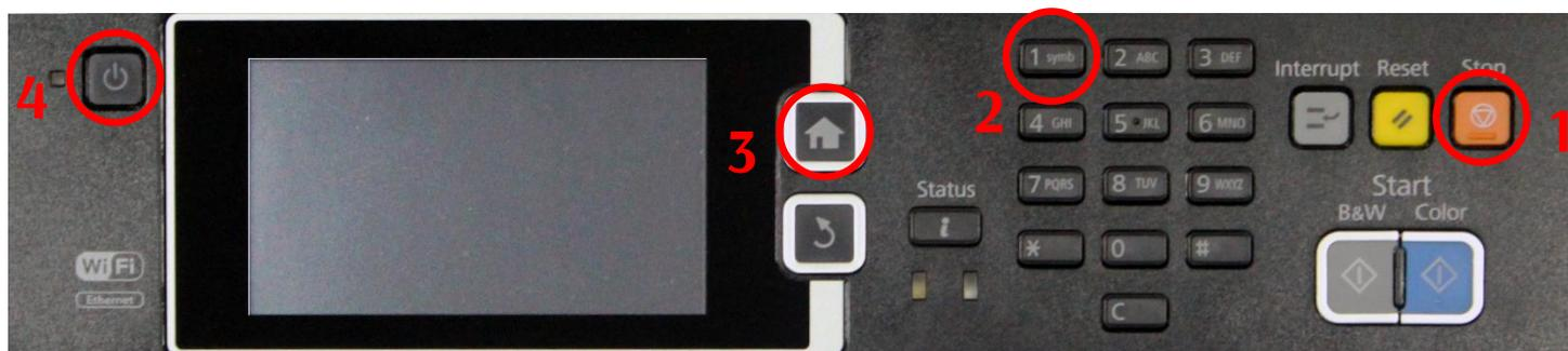
Please note that the inscription on the display must be in white font. If the text is red, this is an incorrect mode, turn off the printer, and then repeat the procedure for entering the printer in firmware mode.
