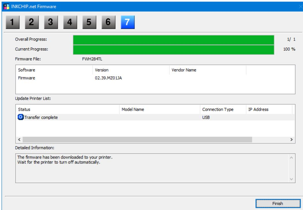
At this point, chipless firmware will be downloaded to the printer. The completion of the download process on to the printer will be indicated by the word “FINISHED” on the printer display. After that, press the “HOME” button on the control panel and the printer will turn off.
